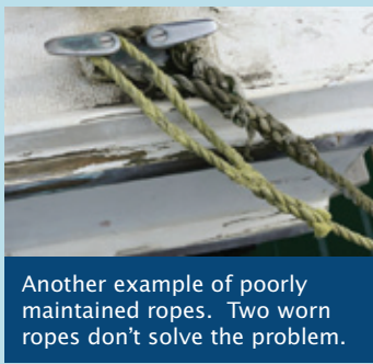
An example of a line that is in poor condition and wearing on the stern of the vessel.
