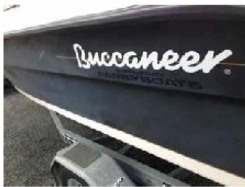
Oxidised gel coat of an 8 year old fibre glass boat.
