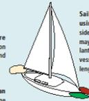
Sailing boats, underway, (not using power) must show sidelights and a stern light. These may be combined into a tri-colour lantern at the top of the mast on vessels less than 20 metres in length.
