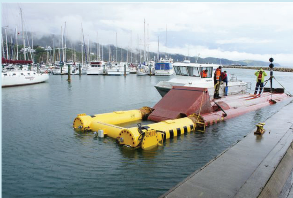
An unusual haul out with the Travelift created a challenge for Mike and Jono recently. A half scale wave generator was towed up to Seaview from the Akaroa Heads and lifted into Unit 2 of the Sea Centre. The wave generator is 18m long and weighs 40 tonnes. As well as this six sea anchors weighing between 2.8 and 4.3 tonnes, a positioning buoy and 4 x 3m mooring buoys are also now residing on our hardstand.
