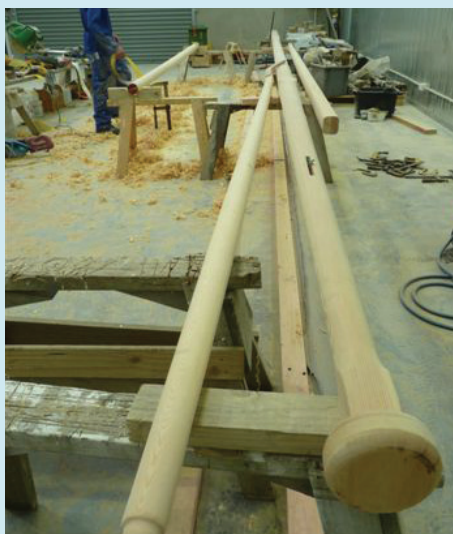
A rare sight these days is the construction of a timber rig. Chris Bowen commissioned Seaview-based boat builder Russell Smith to build a new gaff rig for his Logan 'Spray' in July this year. The work was completed under cover in Sea Centre, Unit 6. Pictured are images of Russell sanding the mast and gaff prior to varnishing. Russell will setting up a workshop in the Sea Centre in January 2012.
