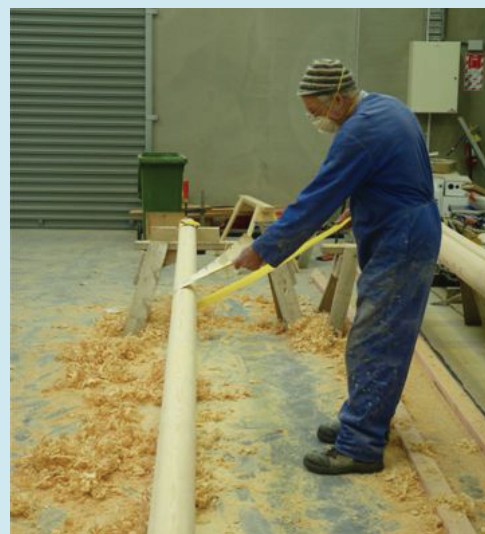
A rare sight these days is the construction of a timber rig. Chris Bowen commissioned Seaview-based boat builder Russell Smith to build a new gaff rig for his Logan 'Spray' in July this year. The work was completed under cover in Sea Centre, Unit 6. Pictured are images of Russell sanding the mast and gaff prior to varnishing. Russell will setting up a workshop in the Sea Centre in January 2012.
