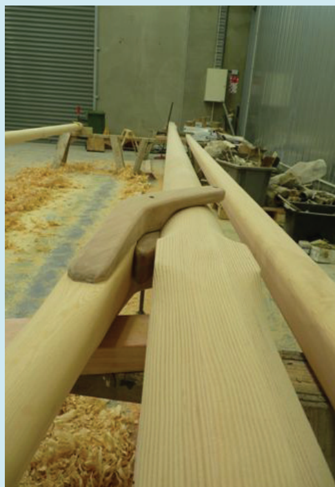
A rare sight these days is the construction of a timber rig. Chris Bowen commissioned Seaview-based boat builder Russell Smith to build a new gaff rig for his Logan 'Spray' in July this year. The work was completed under cover in Sea Centre, Unit 6. Pictured are images of Russell sanding the mast and gaff prior to varnishing. Russell will setting up a workshop in the Sea Centre in January 2012.
