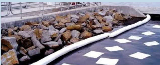
Absorbent pads and booms from a spill kit shown here in use containing and collecting a marina spill
