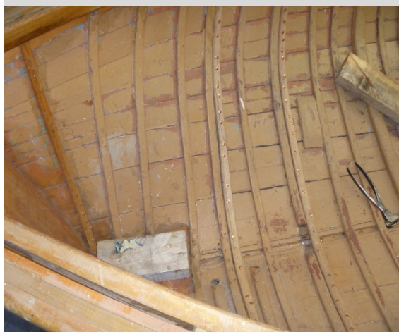
The image above shows two newly inserted ribs, fastened with copper nails, alongside existing ribs. For those of you wondering, as I did, why the nails aren't in a straight line — to do so would risk causing a split in the ribs.
