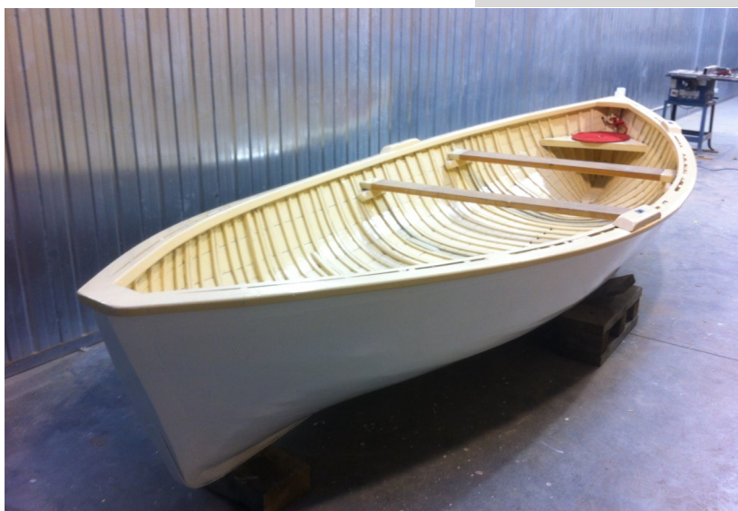
The finished dinghy featuring a few new ribs and a re-caulked hull and freshly painted hull and interior.
