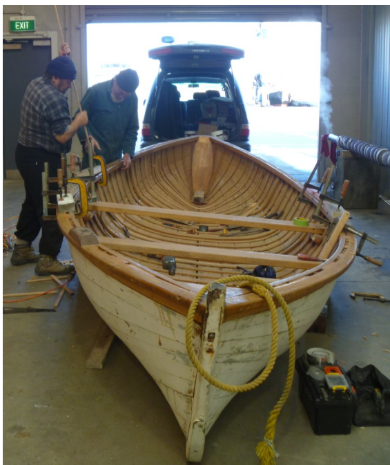
Jim and Russell about to insert a rib—note the steam coming out of the steam box on the right by the shed door.
